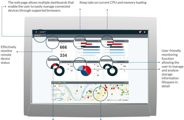
By analyzing the read/write behavior of connected storage devices, iCAP can accurately predict remaining storage device lifetime
