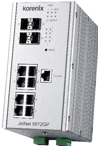
The JetNet 5612GP-4F is an pure Gigabit industrial Ethernet Switch with 8 ports RJ-45, 4 ports Gigabit SFP socket for optical fiber network connection. It adopts high efficiency Ethernet MAC controller with 24Gbps Switch fabric bandwidth, 9K jumbo frame forwarding. The robust system design makes the JetNet 5612GP-4F survive under harsh outdoor environment with extreme electric magnetic interference and the variation of environment temperature.
