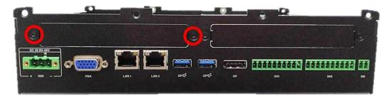
2. Attach the PCI / PCIe Card Installation Kit on, and fasten the two screws back on rear panel to fix the Kit.
