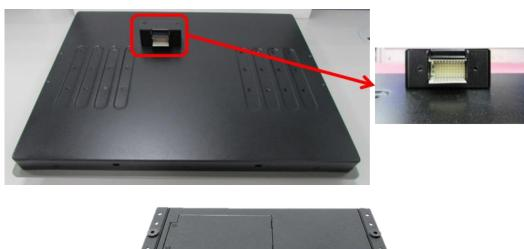
6. Place the P2100 on the display module through its display connector hole as indicated.
