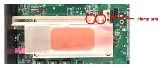
9. Slide the clamp arm of retention module until it contacts the edge of PCI(e) expansion card.
