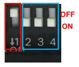
Default setting of Pin1 to Pin4 is OFF/ON/ON/ON.
