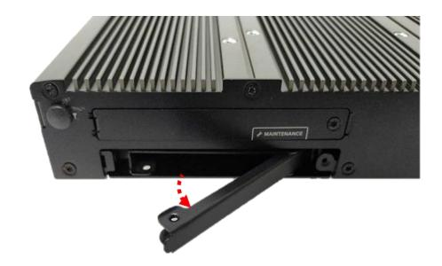
4. Hold the rotating arm to pull out the HDD bracket.
