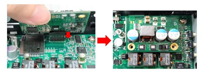
6. Put on the PoE thermal block and fasten two screws to secure the PoE board.
