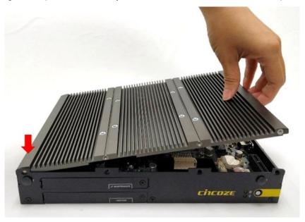
2. Fasten the eight screws at front and rear panel to secure the top cover.
