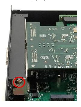
7. Locate the retention module of PCI(e) expansion card.
