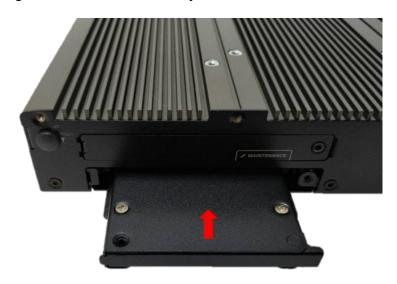
7. Put back HDD bay cover at front panel, and fasten it with the screw.
