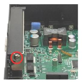
4. Align the notch of golden fingers of Riser card(Optional) with the slot. Insert the card vertically, and press the card straight down into the slot until it's seated firmly.
