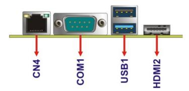
Figure 3-17: External Peripheral Interface Connector
