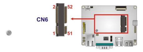
Figure 3-11: PCIe Mini Card Slot Location
