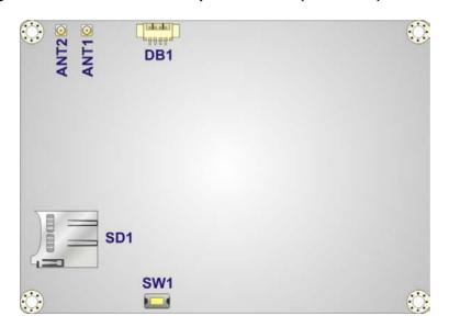
Figure 3-2: Connector and Jumper Locations (Solder Side)
