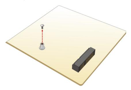
Figure 4-1: Removing the Retention Screw
