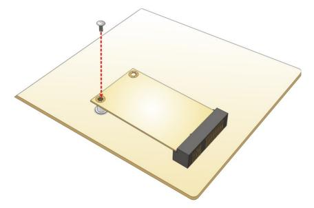
Figure 4-3: Securing the Full-size PCle Mini Card
