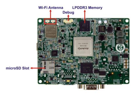
Figure 1-3: Connectors (Solder Side)
