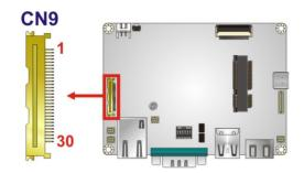
Figure 3-8: eDP Connector Location
