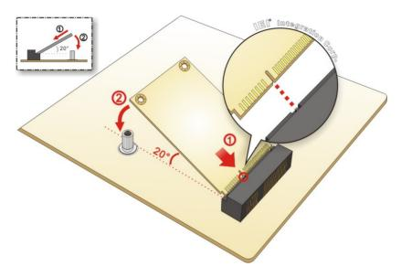
Figure 4-2: Inserting the Full-size PCle Mini Card into the Slot at an Angle
