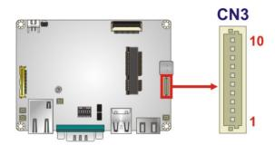
**Figure 3-7: Earphone Connector Location**
