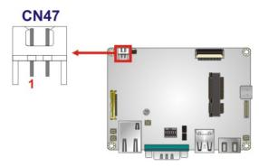
**Figure 3-12: Power Connector Location**
