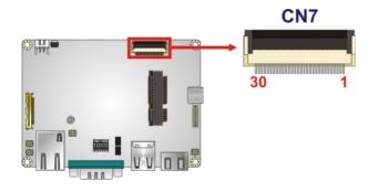
**Figure 3-5: Camera Connector Location**
