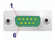
Figure 3-20: Serial Port Pinouts
