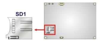
Figure 3-10: microSD Slot Location
