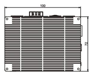
Figure 1-4: Dimensions (mm)
