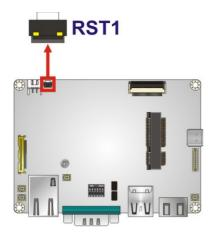
Figure 3-15: Reset Button Location
