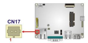
**Figure 3-13: Power Button Connector Location**
