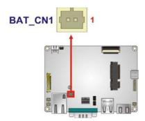
Figure 3-4: Battery Connector Location
