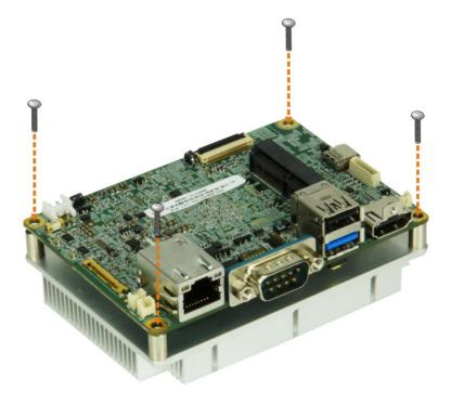
Figure 4-4: Heat Sink Installation
