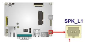
**Figure 3-16: Speaker Connector Pinouts**
