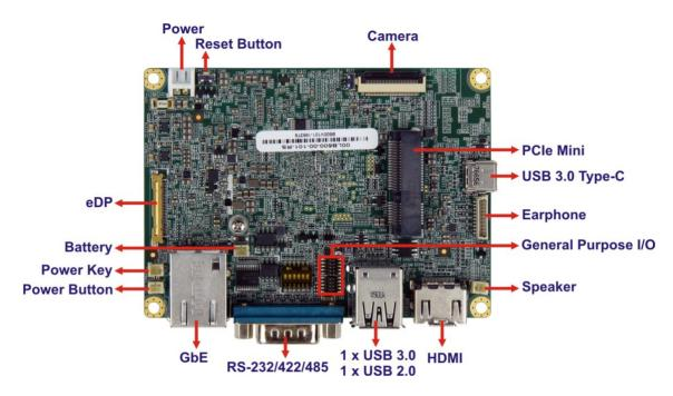
Figure 1-2: Connectors (Front Side)
