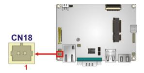
Figure 3-14: Power Key Connector Location
