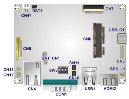
Figure 3-1: Connector and Jumper Locations (Front Side)
