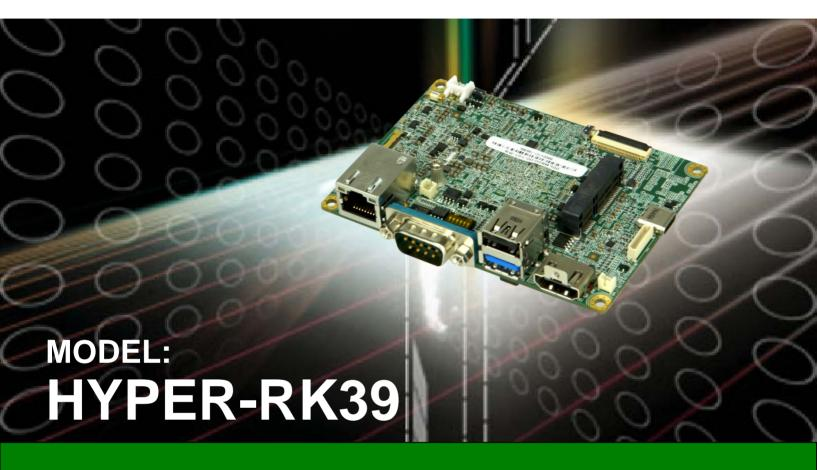
Pico-ITX SBC with Rockchip RK3399 Processor, 2 GB LPDDR3, 16 GB eMMC Flash, HDMI, eDP, GbE LAN, PCle Mini, USB 3.1, USB 2.0, COM and RoHS
