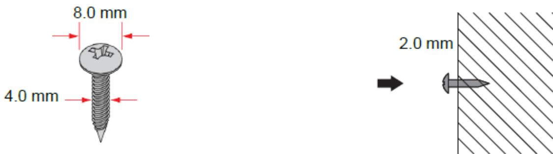
**Figure 2.5 Securing Wall Mounting Screws**
