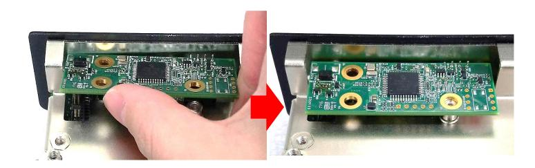
2. Fasten a screw to fix the CFM-IGN Module.
