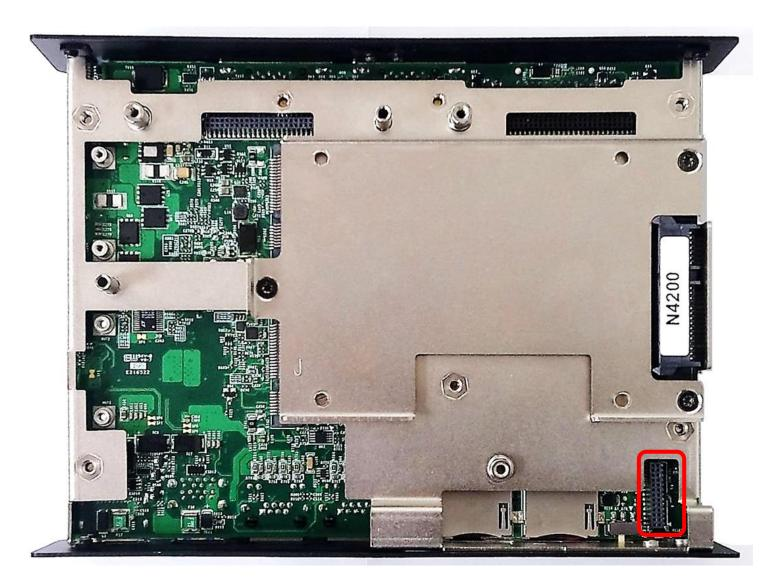
Locate the CFM-IGN Module's connector on system motherboard as indicated.
