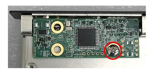
1. Locate the PoE connector on system motherboard as indicated in page 76, and insert the female connector of CFM-PoE module to the male connector on system's mainboard.
