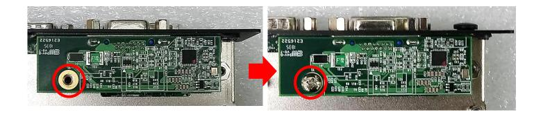
6. Attach the CMI-DVI bracket, and fasten 2 screws as marked.
