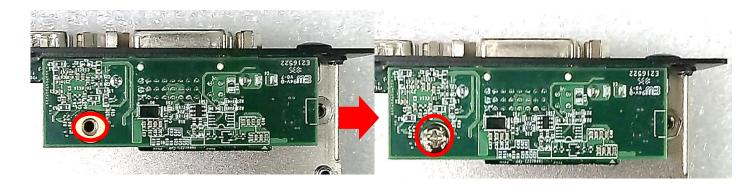
6. Attach the CMI-DVI bracket, and fasten 2 screws as marked.
