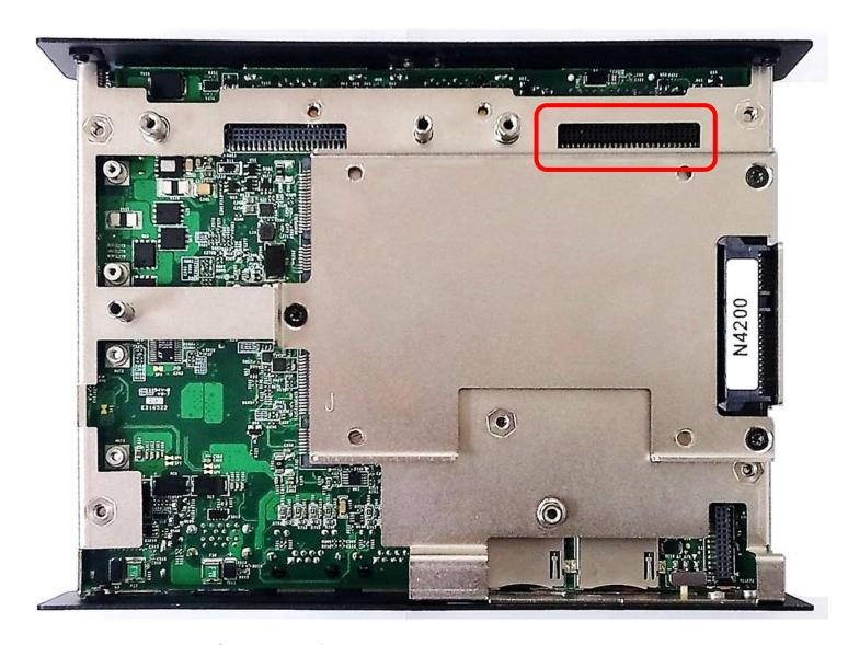
Locate the CMI Modules/ connectors on system motherboard as indicated.
