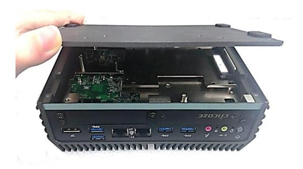
2. Fasten the 4 screws to fix the cover.
