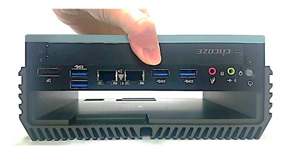
1. Level the grooves on the cover at front and rear panels. Put on the cover.
