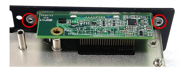
4. Push the connector pins on CMI-VGA module until the pins can be inserted completely to the female connector (BTB\_FH1) on the system's mainboard.
