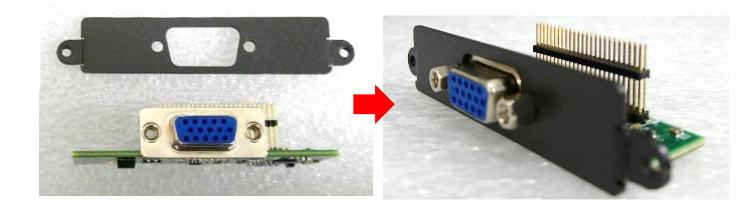
3. Align two holes on the CMI-VGA bracket with the holes on the rear panel.
