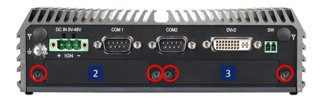
2. Attach the CMI-DIO bracket on the backside of system's rear panel, and fasten it with two screws.
