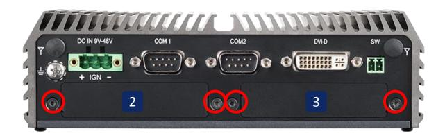
2. Assemble the CMI-COM bracket and CMI-COM module together with 4 D-Sub jack screws
