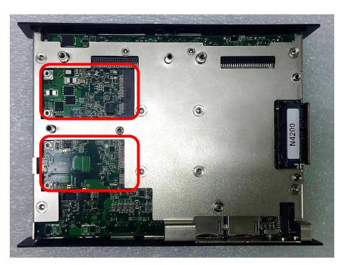
3. Tilt the Mini PCIe modules at 45 degrees angle and insert it to the slot until the gold-pated connector of module contacted firmly with the slot.
