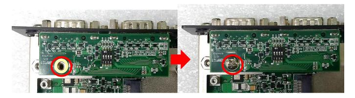
6. Fasten 2 screws for each CMI-COM bracket as marked.
