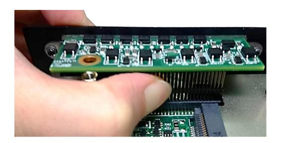
4. Make sure the hole on CMI-DIO module is aligned with the screw hole on the system's mainboard, and fasten a screw to fix it.
