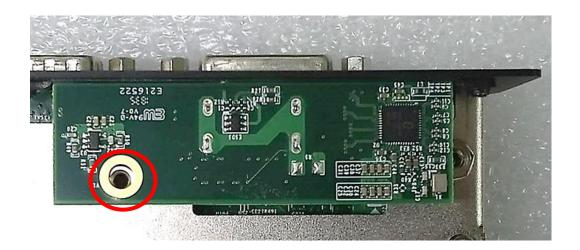
4. Fasten a screw to fix the CMI-HDMI module.
