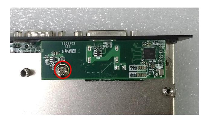
5. Align the hole on CMI-HDMI module with the screw hole on the system's mainboard module, and insert vertically to the female connector (BTB\_FH1) on the system's mainboard.
