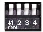
Default setting of Pin1 to Pin4 is OFF/ON/ON/ON.
