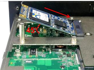
4. Press down the module and use two screws to fix a module.
