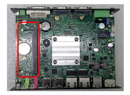
2. Tilt the SODIMM module at a 45 degree angle and insert it to SODIMM socket until the gold-pated connector of module contacted firmly with the socket.
