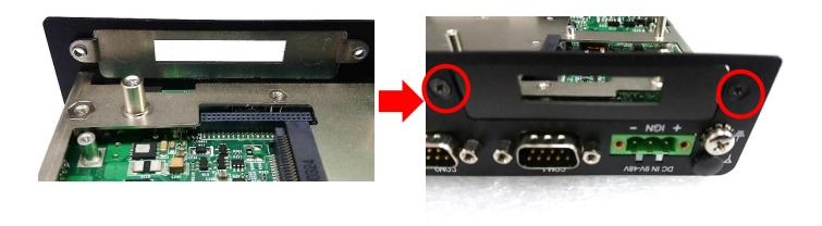
3. Push the connector pins on CMI-DIO module until the pins can be inserted completely to the female connector (BTB\_FH2 or BTB\_FH1) on the system's mainboard.
