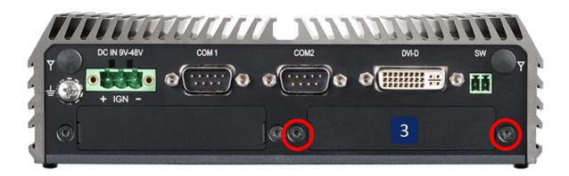
2. Attach the CMI-HDMI bracket on the backside of system's rear panel, and fasten it with two screws.
