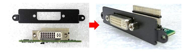
3. Align two holes on the CMI-DVI bracket with the holes on the rear panel.
