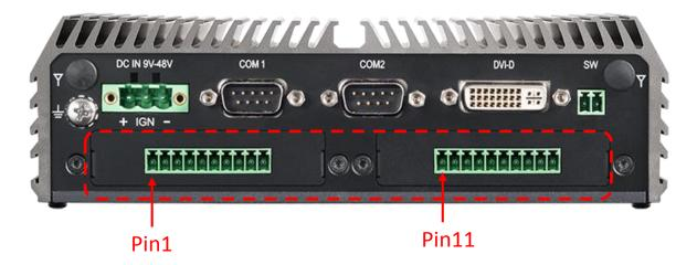
**DIO1: Digital Input / Output Connector**Connector Type: Terminal Block 2X5 10-pin, 3.5mm pitch
