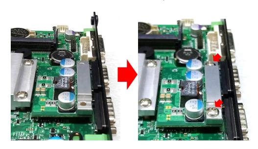
4. Paste the thermal pads onto the heatsink and coil carefully.
