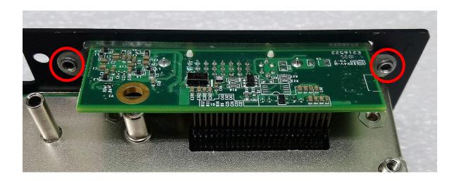
4. Push the connector pins on CMI-DVI module until the pins can be inserted completely to the female connector (BTB\_FH1) on the system's mainboard.
