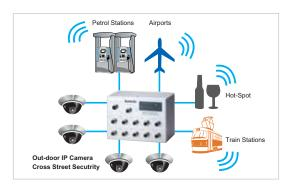
120W per unit at 60°C operating. temperature, to drive the motors of outdoor PTZ IP cameras with direction control for cross–street monitoring, or WiMAX systems for internet access in train stations, airports or Hot-spots.
