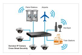
power mode (at 50°C) to outdoor PTZ IP cameras with direction control for cross–street monitoring, or WiMAX systems for internet access in train stations, airports or Hot-spots. The additional dual Gigabit ports provide more resilient and redundancy for users while forming a ring network and delivering increased bandwidth to the central network.
