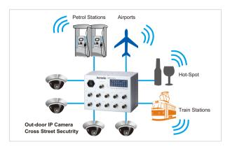
200W per unit at 60°C op. temperature, to drive the motors of outdoor PTZ IP cameras with direction control for cross-street monitoring, or WiMAX systems for internet access in train stations, airports or Hot-spots.
