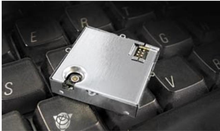
*Lassen SQ GPS receiver with metal shield*
