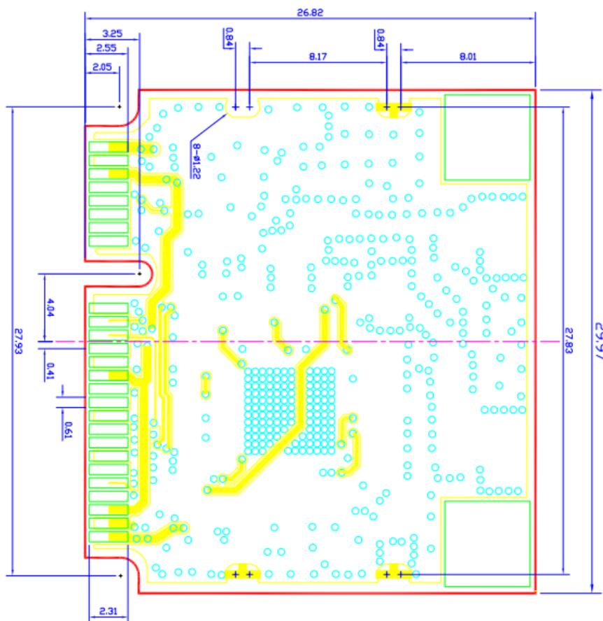
Figure 1-2: WIFI-RT3593-DB Dimensions (mm)
