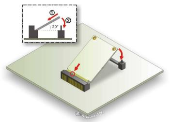
**Step1. Insert into the socket at an angle**. Line up the notch on the card with the notch on the connector. Slide the IVCME-C604 into the socket at an angle of about 20°.
