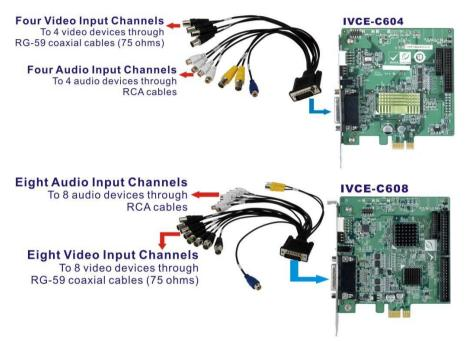
Step1. Align and insert the DB-26 male connector from the cable to the
