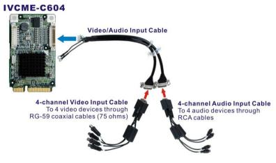
**Step1.** Align and insert the wafer connector from the video/audio input cable to the 10-pin wafer connector (CN1) on the board.
