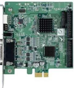
**Step1.** Align and insert the DB-26 male connector from the cable to the DB-26 female connector on the board.
