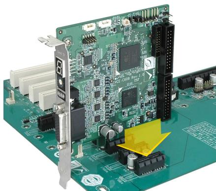
**Step4.** Insert a retention screw through the top of the video capture card external bracket into the chassis to secure the card to the chassis.
