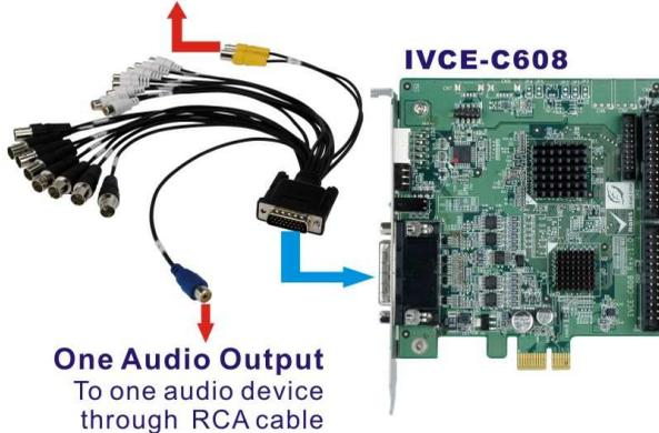
**Step1.** Align and insert the DB-26 male connector from the cable to the DB-26 female connector on the board.
