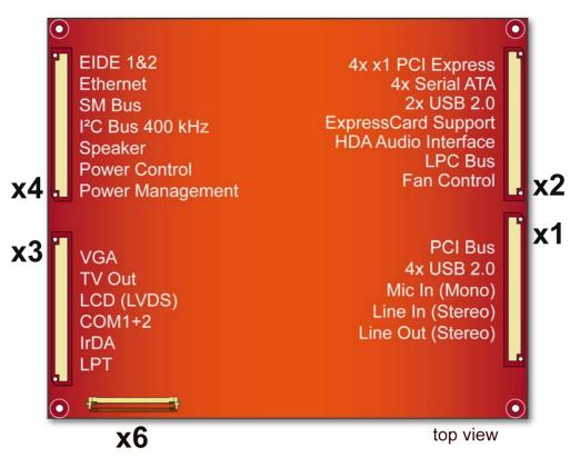
In this view the connectors are seen "through" the module.
