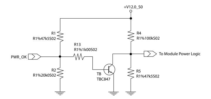
The voltage divider ensures that the input complies with 3.3V CMOS characteristic and also allows for carrier board designs that are not driving PWR\_OK. Although the PWR\_OK input is not mandatory for the onboard power-up sequencing, it is strongly recommended that the carrier board hardware drives the signal low until it is safe to let the module boot-up.
