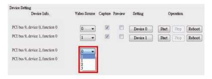
**Step5.** This step is only required for the HDC-304E. Select the transmitter bus from 0 to 3. For example, to view the video input source 1 on HDMI display device, select the transmitter bus 0. Please refer to the following table:
