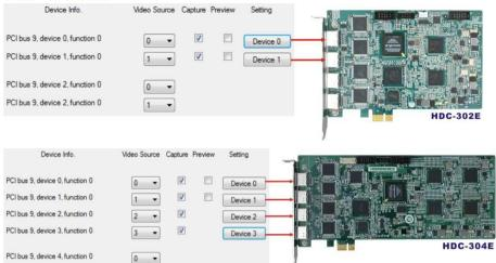
**Step3.** Click the Device # button. The Encoding window appears. Choose the video input format which depends on the video device. **The video format selected here must be same with the HDMI input video format.** The available options include:
