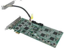
**Step4.** Secure the HDMI port bracket to the system chassis.
