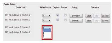
**Step7.** This step is only required for the HDC-304E. Select the transmitter bus from 4 to 7. For example, when the Device0 button is selected to decode the encoded file, please select 4 from the device4 (transmitter bus) drop-down menu to display the video on HDMI display device by output kit. Please refer to the following table:
