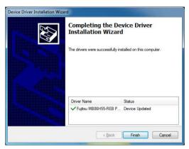
**Step8.** Check the device manager in the Windows control panel to ensure the driver (MB86H55-REB PCI, HDC controller and WinDriver) has been properly installed. The installed driver is slightly different on different models.
