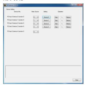
**Step2.** Enable and configure the device settings by clicking the Device # (0, 1, 2, 3) buttons. The device number is decided by which port the device is installed. If the HDC-301 series is installed, there will be only one Device 0 button to choose.
