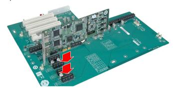
**Step4.** Insert a retention screw through the top of the video capture card external bracket into the chassis to secure the card to the chassis.
