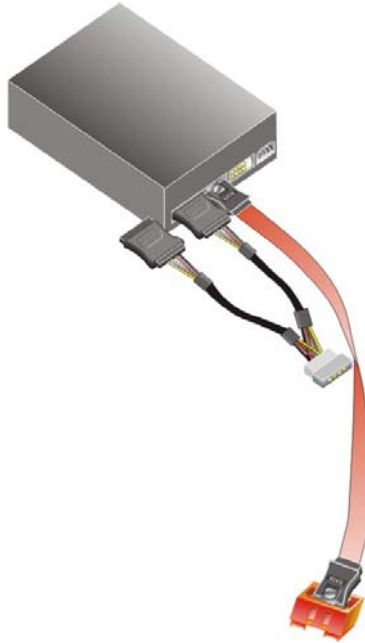
Figure 5-13: SATA Power Drive Connection
