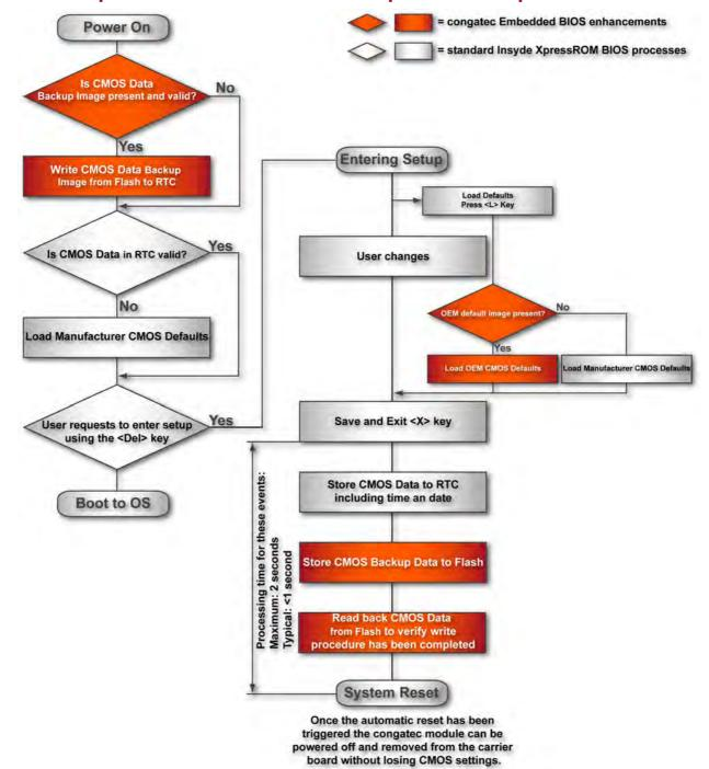
The above diagram provides an overview of how the BIOS Setup Data is backed up on conga-XLX.
