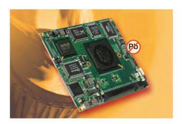
AMD Geode™ LX processors with an AMD Geode™ CS5536 companion device
