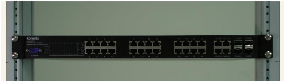
When installing multiple switches, mount them in the rack one below the other. It's requested to reserve 0.5U-1U free space for multiple switches installing. This is important to disperse the heat generated by the switch.
