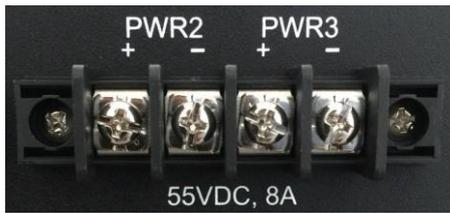
1. Insert positive and negative wires into V+ and V- contacts respectively of the terminal block connector.
