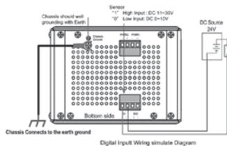
**Note: The DI accepts DC type signal and supports isolated input circuit with Digital High Level input DC 11V~30V and Digital Low Level input DC 0V~10V.**
